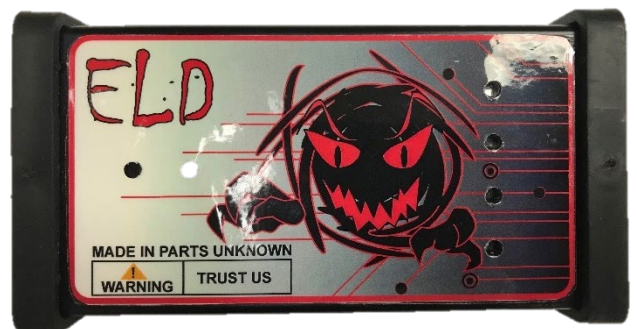
Figure 11: A compromised vehicle diagnostics adapter (VDA)
